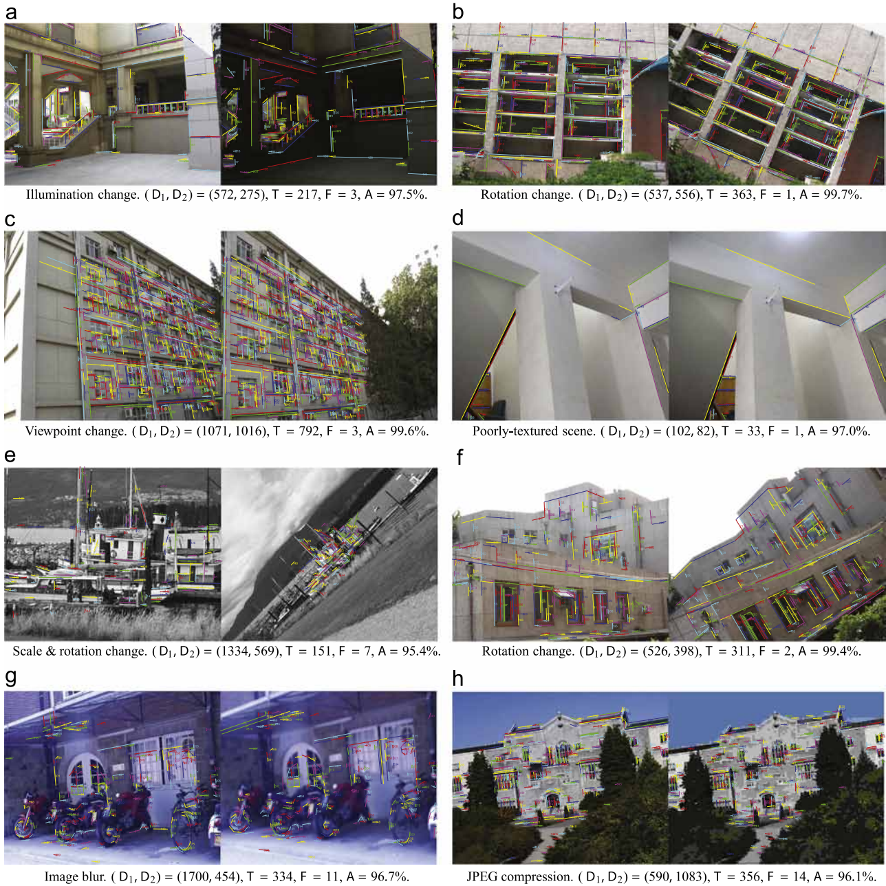
Fig. 12. The line matching results of the proposed method on eight representative image pairs. We will refer the eight image pairs as (a)–(h) for later use. In the caption of each subfigure, (D_1, D_2) denotes the pair of numbers of the extracted line segments in the two images. T represents the number of total matches found by the proposed method between the two sets of line segments extracted from the two images. F and A denote the number of false matches among the total matches and the corresponding accuracy, respectively. Two line segments in correspondence from a pair of images are drawn in the same color and are labeled with a same number at the middles. (For interpretation of the references to color in this figure caption, the reader is referred to the web version of this paper.)
