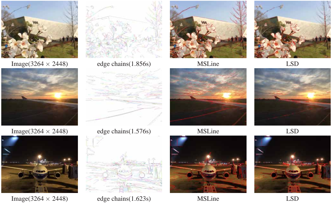
Figure 7. Comparison between the LSD and the line segments detector formed by combining the proposed MSEdge and the Least Square Fitting method on three large size images captured by a smart phone.
