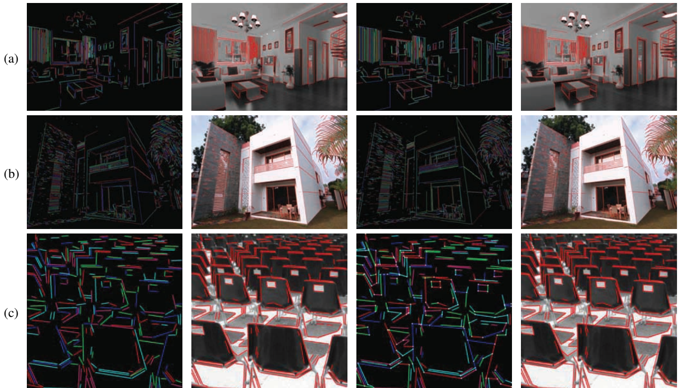
Fig. 6. Experimental result on three different kinds of scenes. The four columns from left to right are: the line segments detected by EDLines, the overlapped image of EDLines, the line-networks recovered by NETLines, the overlapped image of NETLines. In (a) the number of line segments detected by EDLines is 518 with a total line length of 22105.5 in pixels, these of NETLines are 469 and 24157.7. In (b) these figures are 1821 and 66192.2 for EDLines, 1697 and 72027.4 for NETLines. In (c) these figures are 305 and 6425.0 for EDLines, 302 and 6962.5 for NETLines.
