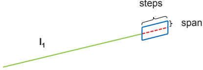
Fig. 2. Searching step and span: The searching steps of the line segment l_1 is set as 1/10 of its length, and the searching direction of l_1 is converted into the vertical.
