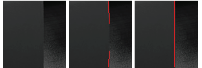
Fig. 5. Precision comparing between the result of EDLines and NETLines: from left to right are the original image, the overlapped image of the line segments detected by EDLines on the original image, and the overlapped image of the refined line segments on the original image.
