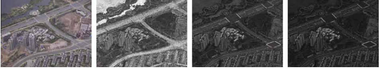
Fig. 1. An original aerial image (Left) and its normalized texture complexity maps with different values of \delta ( \delta = 0, 4, 8 from the second column to the last) where the lighter regions indicate higher texture complexities.
