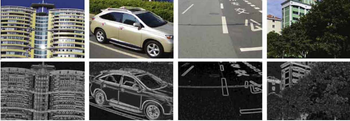
Fig. 2. The four typical regions (Top) in street-view panoramic images and their corresponding normalized texture complexity maps (Bottom) where the lighter regions indicate higher texture complexities.
